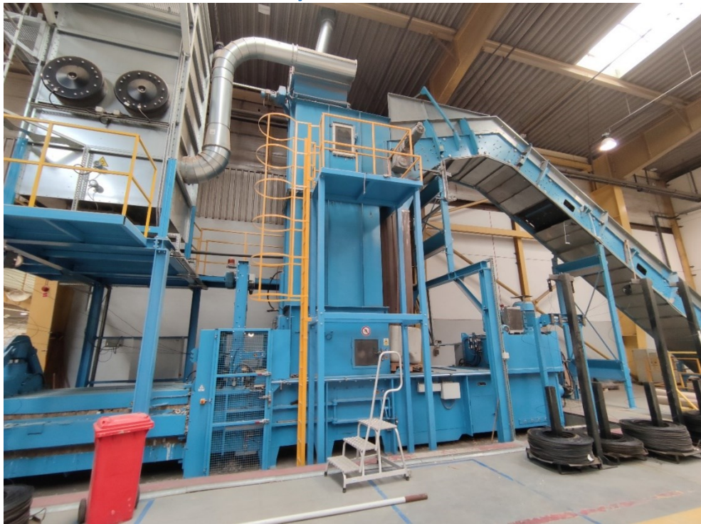
Figure E5-0-1. Paper waste packaging machine at Schumacher Packaging Sp. z o.o.
